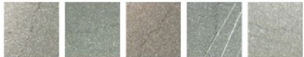
(a) Tiny cracks with low contrast and different brightness.
